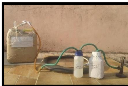
Fig. No. 3: Anaerobic Digester
